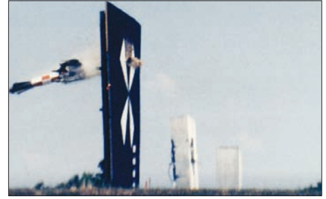
The US Air Force EDGE High Gear program trialled an extremely accurate Wide Area Differential GPS scheme for weapons guidance. Depicted images from drops of modified GBU-15 glidebombs, using only differential GPS guidance.
