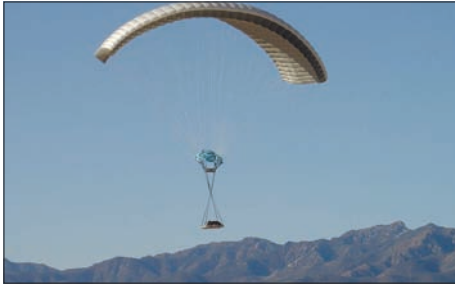
The Joint Precision Airdrop System (JPADS) uses GPS and steerable parachutes to provide extremely high accuracy compared to traditional airdrop deliveries.
