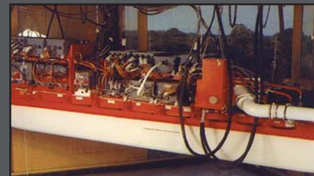
The Grumman/Norden and Hughes Pave Mover demonstrators proved the concept of highly accurate DPCA GMTI radar. Both were carried in the weapon bay on an F-111E (Norden).
