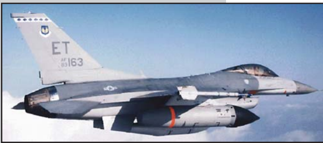
The Norden APG-76 MMRS was the first fighter radar to employ DPCA GMTI capability, providing exceptional tracking accuracy. (Northrop-Grumman)
