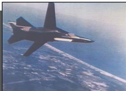
The Grumman/Norden and Hughes Pave Mover demonstrators proved the concept of highly accurate DPCA GMTI radar. Both were carried in the weapon bay on an F-111E (Norden).
