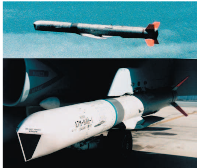
The SLAM-ER is the ultimate evolution of the Harpoon, using a Tomahawk derived warhead, GPS/inertial midcourse guidance, and a datalink system for man-in-the-loop terminal guidance, exploiting a nose mounted thermal imaging seeker. The SLAM-ER is the most mature of the FOSOW contenders, but is likely to be supplanted in US Navy service by the JASSM as the latter matures (Boeing).
